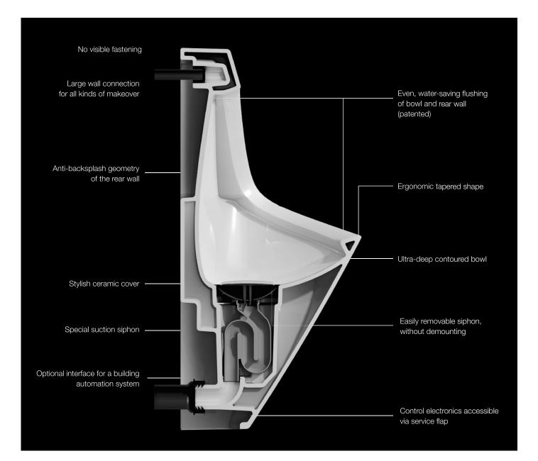
LAUFEN urinals are set to revolutionise the upkeep and maintenance of public sanitary facilities. Up till now, urinals often had to be completely disassembled when replacing their siphons. antero and lema allow you to release the siphon easily using a special key and lift it out.
