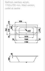
2**2350.1** Bathtub, sanitary acrylic, 1700x750 mm, fitted version, with frame, also available with whirl system
