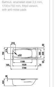
2**2511.3**.040 Bathtub, enameled steel 3,5 mm, 1700x750 mm, fitted version, with anti-noise pads, with holes for handles
